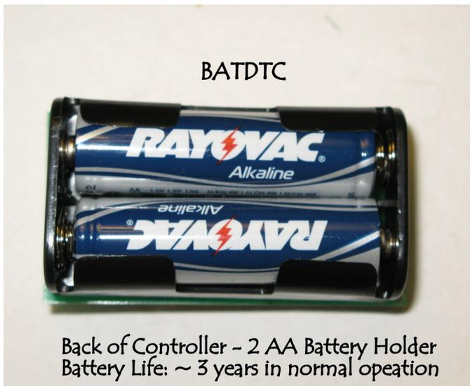
**Ambient Temperature Range:** The BATDTC will operate from -25F - 158F.
